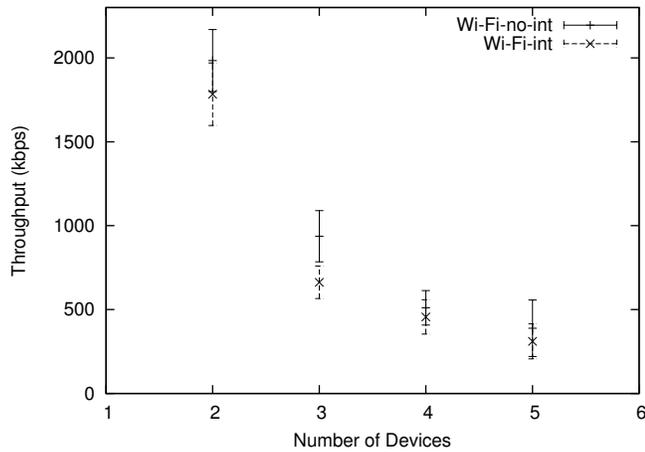
Fig. 3. Wi-Fi throughput with and without interference
