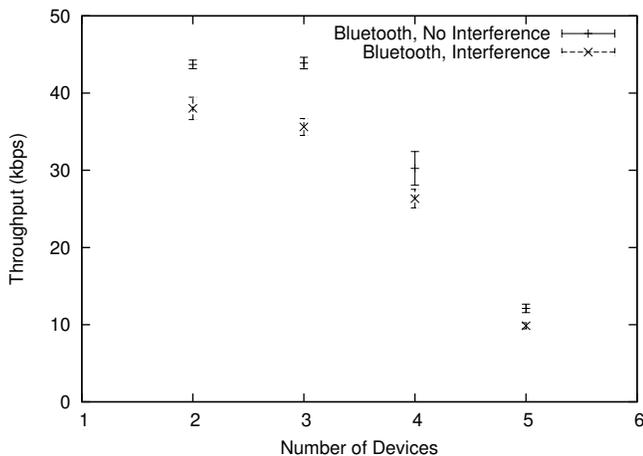
Fig. 2. Bluetooth throughput with and without interference
